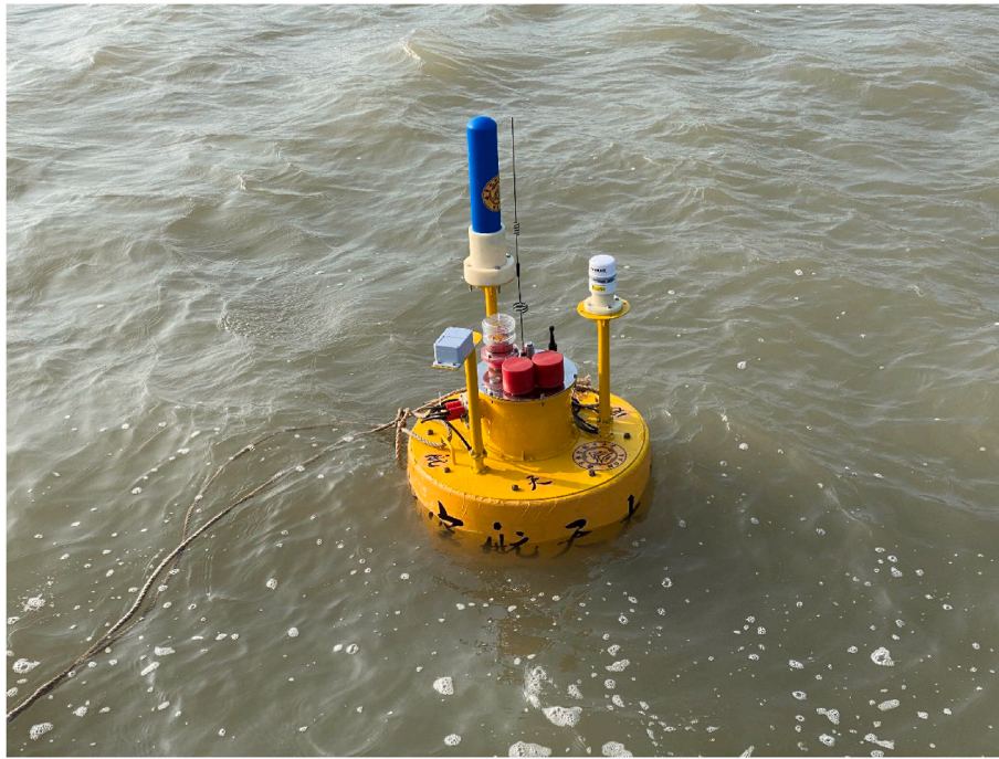
Fig. 10. The marine radioactivity online monitoring system working in the seawater.
