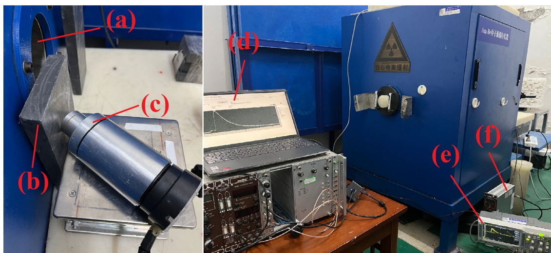
Fig. 3 Experimental equipment. a ^{241}\text{Am-Be} neutron source. b Lead plate. c CLYC detector. d Upper computer. e Oscilloscope. f High voltage power supply
