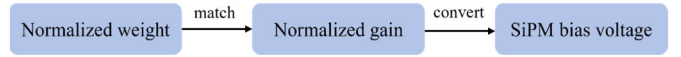
Fig. 3. Establishment of the relationship between weight of the encoder and SiPMs' bias voltage.
