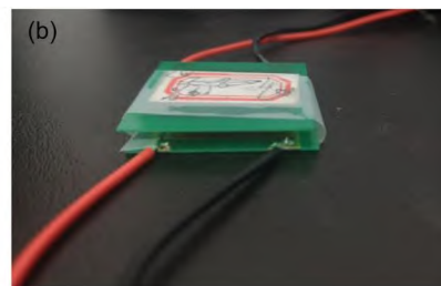
图 12 叠层氚基同位素电池的结构模型(a)及实物图(b) Fig.12 Structural model (a) and physical diagram (b) of stacked tritium-based nuclear battery
