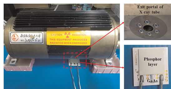
Figure 14. Prototype of the experimental set up enhanced by the phosphor layer.
