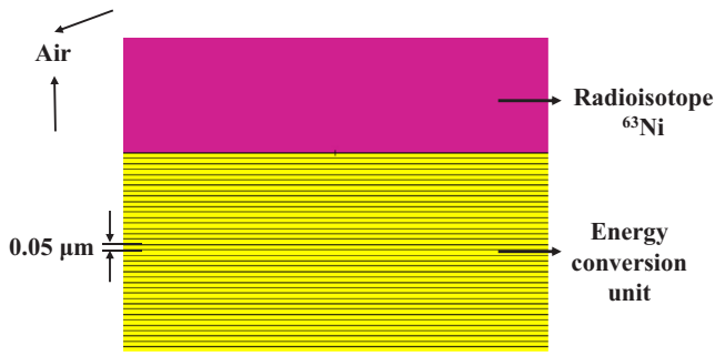
Fig. 1. Calculation monolayer model of 63 Ni-Si betavoltaic microbattery used to study the temperature dependence using MCNP5.
