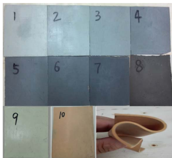
Figure 1. Flexible X-ray-shielding VMQ composite samples. [Color figure can be viewed in the online issue, which is available at wileyonlinelibrary.com.]
