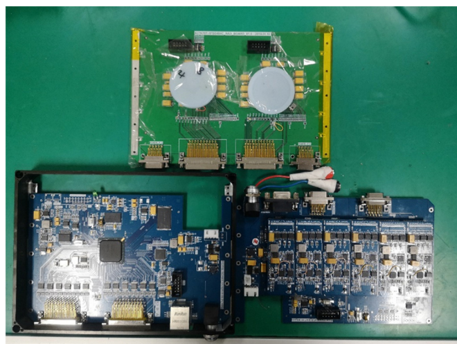
Fig. 2. Control, power and irradiation boards of the FPGA test system.
