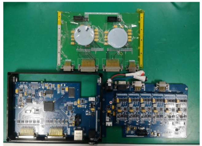
Fig. 2. Illustration of the irradiation board and the test system hardware.
