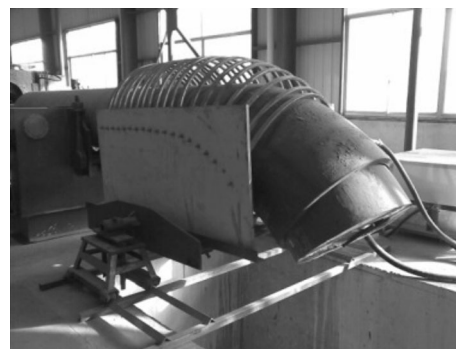
Fig. 9 Equipment of hot push bending process
