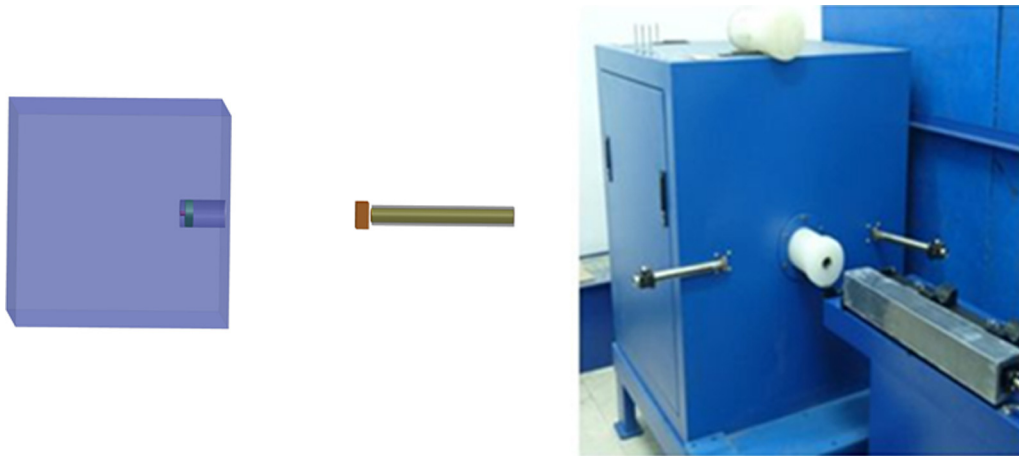
Fig. 5. The MCNP geometric model and a photo of the neutron detection equipment.
