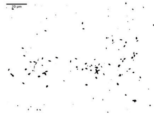
Fig. 6. Optical image (60x) of tracks left on the CR-39 by alpha and lithium ions coming from the neutron capture reaction on ^{10}\text{B} .
