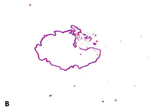
Fig. 5. Optical images (60x) of a flaw on the CR-39 surface, used as ROI to show the accuracy of the re-positioning method. Scheme A is the flaw image. Scheme B is the overlap of the edges of two images taken after re-positioning the CR-39.
